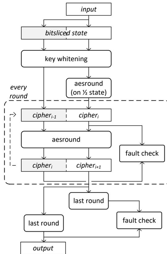
Figure 7.6: Time-Redundant computation of a bitsliced AES
