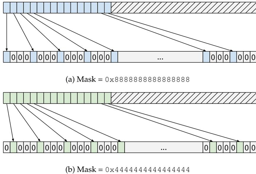
Figure 8.1: Intel `_pdef_u64` instruction
