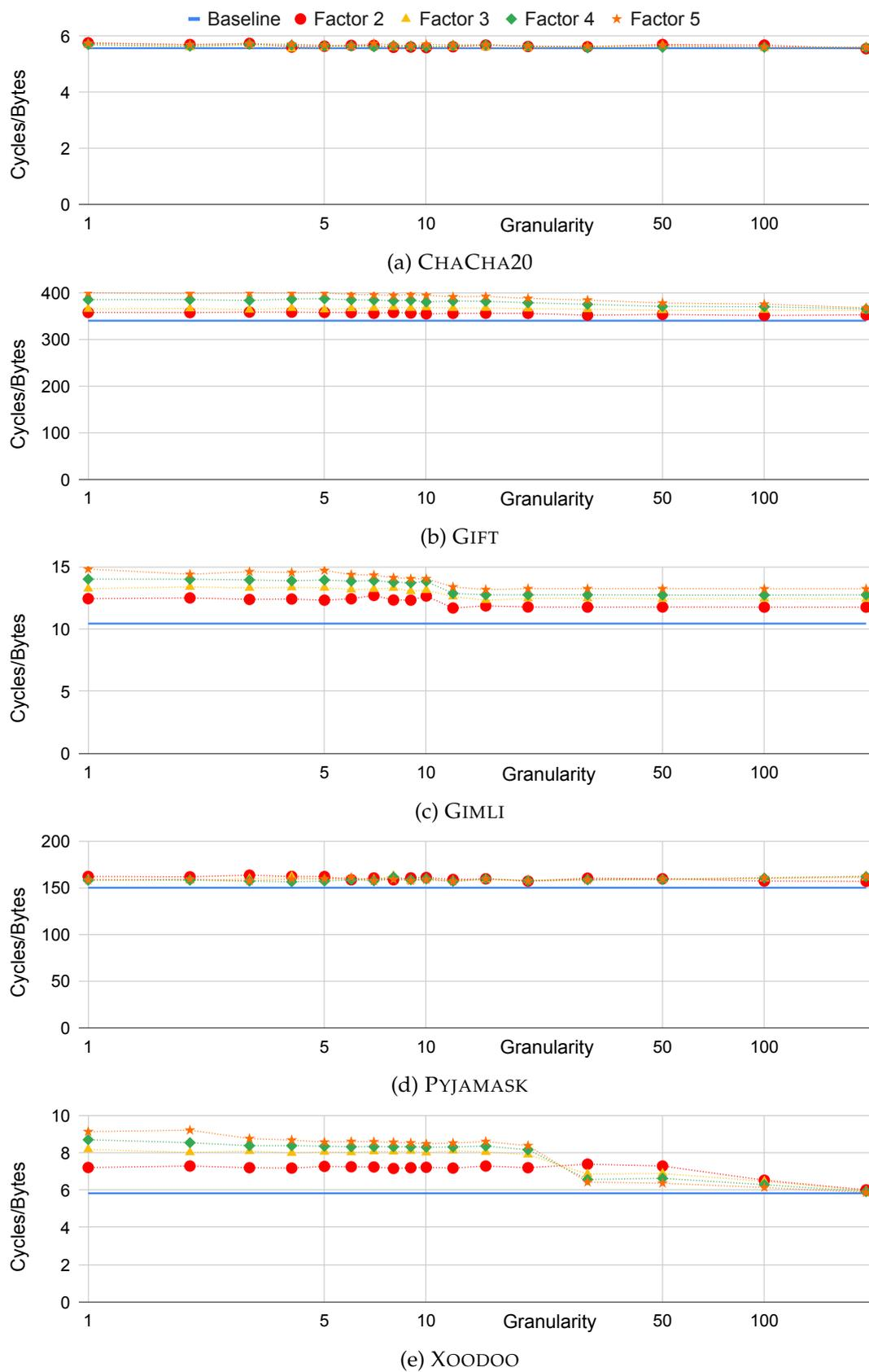
Figure 4.9: Impact of interleaving on general-purpose registers
