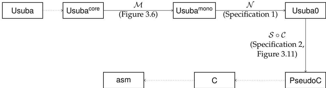
Figure 3.1: Usuba's formal pipeline
