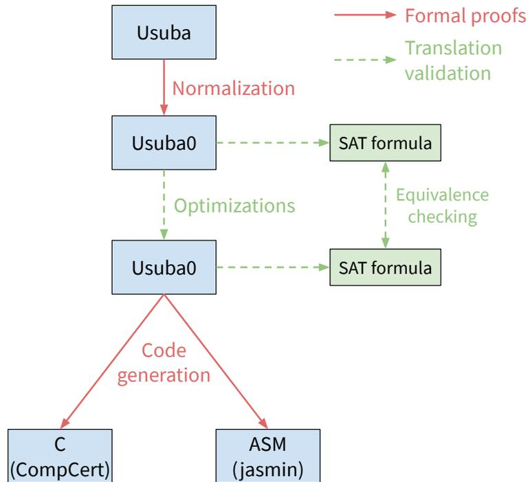
Figure 8.8: Pipeline of a semantics-preserving Usuba compiler
