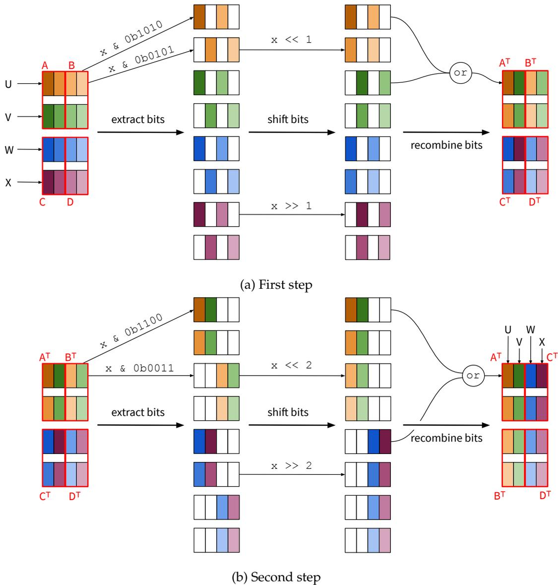
Figure 1.10: Optimized transposition of a  $4 \times 4$  matrix
